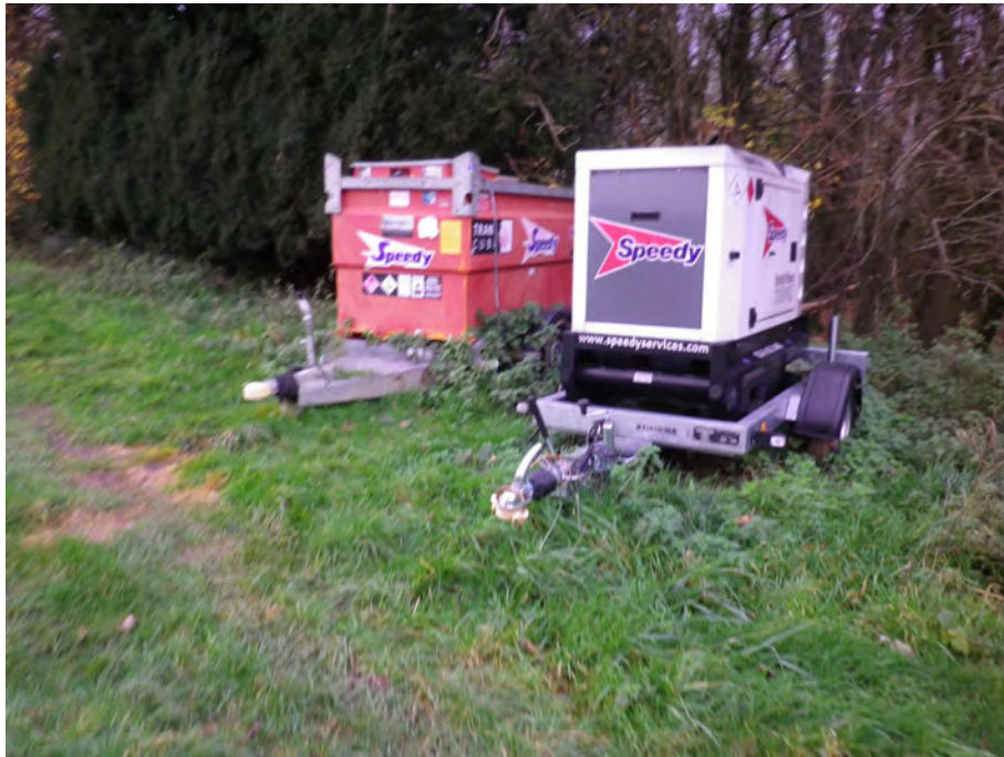
Plate 9 – Photograph showing towable fuel bowser and generator
